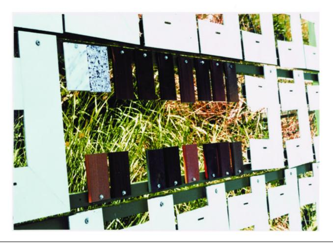
Exposure station for natural ageeing test in Fusina (Venice) Samples made end of 1995 and exposed for 1 year in industrial-marine atmosphere
